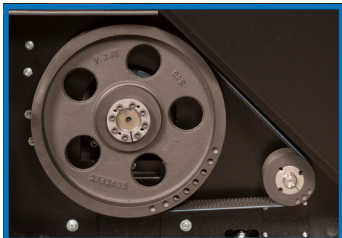
Flywheel-type rotor pulley with taper-lock bushing
