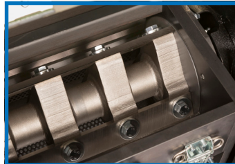
Welded steel rotor with rotating end disks
